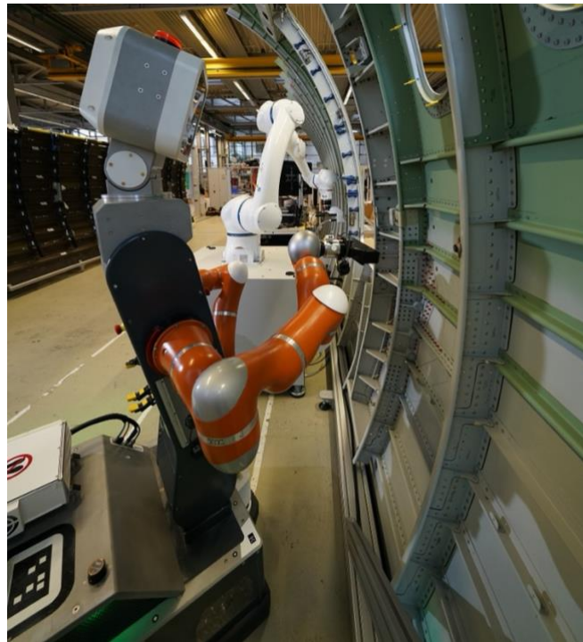
Figure 26: Fraunhofer IFF Swap-IT architecture for aircraft construction
