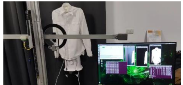
The QUAD-AI@E prototype, a smart inspection station using computer vision to detect garment defects in real-time.
