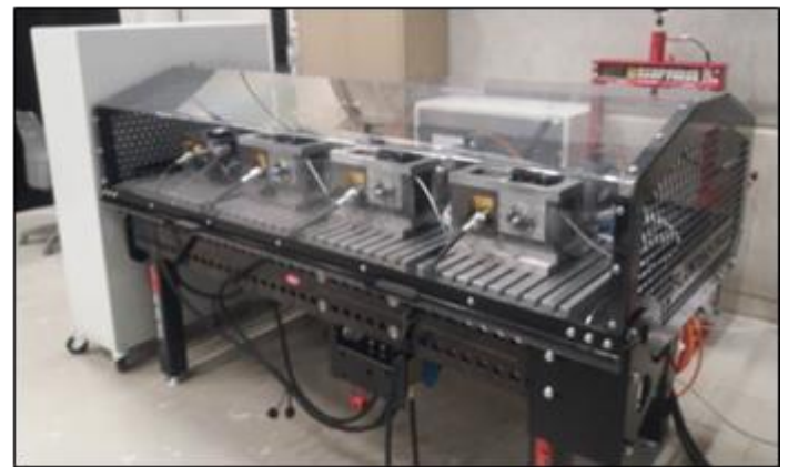
The Didactic Factory setup: a fleet of drivetrains used to simulate faults and train AI models for predictive maintenance.
