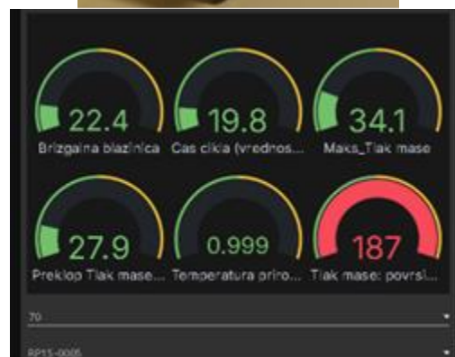
The MouldWatcher edge device: visualizing real-time process parameters directly on the moulding machine.
