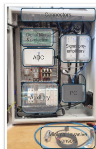
Details of the custom hardware unit and the non-intrusive 'clip-on' sensors used for data collection.
