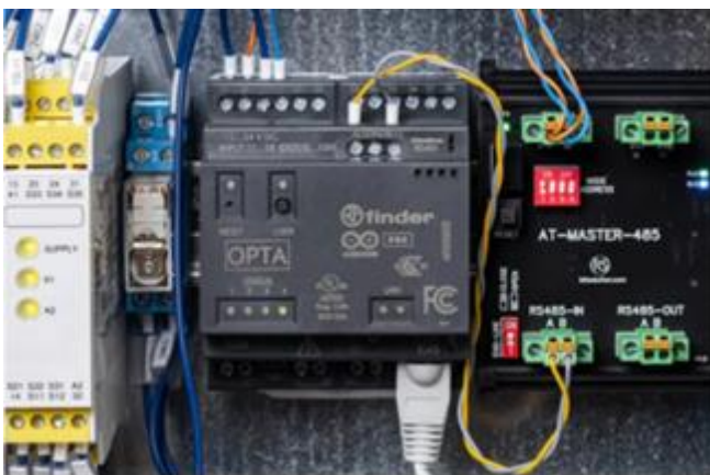
The Arduino-based PLC (Opta) embedded with lightweight neural networks to detect boiling anomalies directly at the source.
