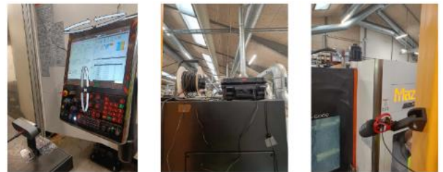
The IoT Suitcase in action: a portable edge device collecting data directly from the production line.
