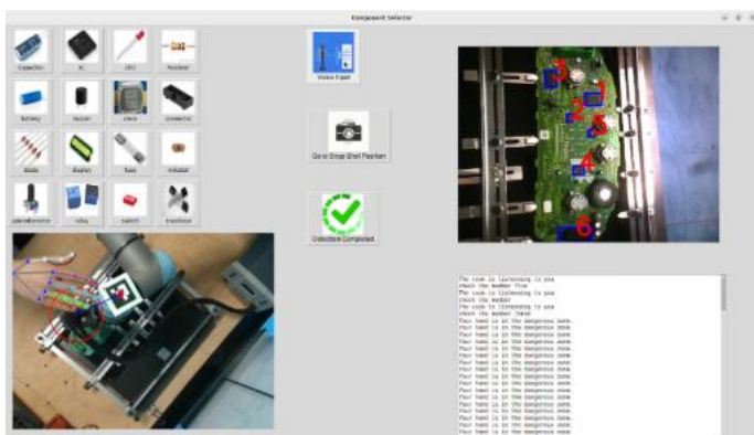
The AI interface, combining computer vision for component detection with voice command feedback.
