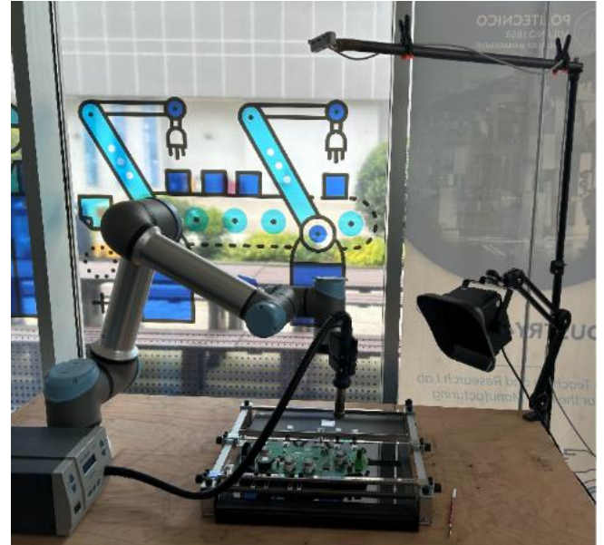
The collaborative workstation, a cobot assists the human operator in disassembling electronic boards safely.
