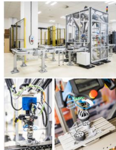
The robotic assembly workstation at CTU Prague, utilizing force-torque sensors for real-time, explainable anomaly detection in dynamic production.
