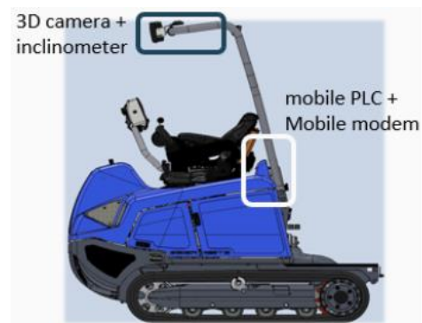
The AGRIDRIVE setup: retrofitting a standard tractor with 3D cameras and inclinometers for smart navigation.
