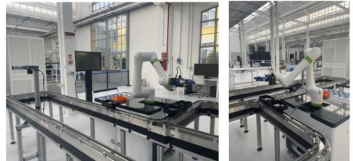
The adaptive workstation: a collaborative robot that adjusts its speed based on the operator's biometric feedback.
